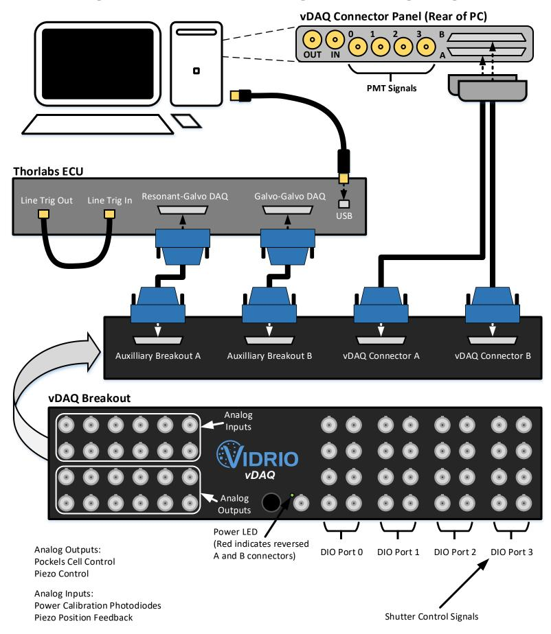
When Auxiliary Breakout A is connected to Resonant-Galvo DAQ, the following channels should not be used: D2.7, AO9, AI9 When Auxiliary Breakout B is connected to Galvo-Galvo DAQ, the following channels should not be used: AO10, AO11, AI10, AI11
